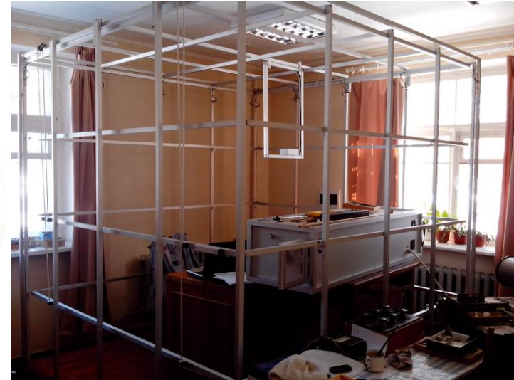
The MMLFC shielded room, where the field is several orders of magnitude smaller than the external one. In the foreground is the device for thermal demagnetization - furnace MMTD
